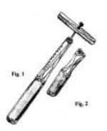
it slightly bigger than the thickness of the headed nail. You can make the hole with a drill, or by hammering a fatter nail through, wiggling it around, and then pulling it out. Mount the propeller onto the notched end of the bugger stick with the headed nail (Fig. 1), but don't drive the nail in all the way. Leave it out just a little so that the propeller spins very easily. If necessary, balance the propeller by carving chips off the heavier end.
